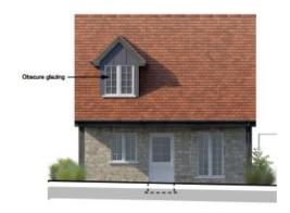
Quoin details would match the surrounding buildings. Traditional lime mortar will be used to match existing buildings in the area. The site would be dug down and the current retaining wall to the land would be removed. All stones form the demolition of both the existing
